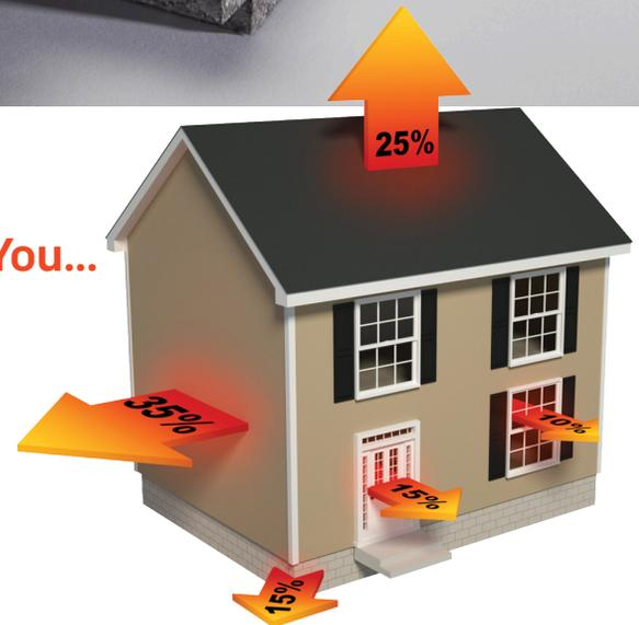
Nearly 25% of your home's wall is made up of studs that typically are not insulated, so it's like having one entire wall of your home with no insulation. Adding insulation to your home's exterior under new siding can help your home meet U.S. Department of Energy (DOE) insulation recommendations, as well as state and local codes.
