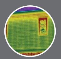
Before Insulation Thermal imaging reveals two energy leaks: yellow lines where energy escapes through studs, and red at the top of the wall where
