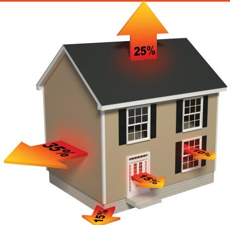
Nearly 25% of your home's walls are made up of studs that typically are not insulated, so it's like having one entire wall of your home with no insulation. Adding insulation to your home's exterior under new siding can help your home meet U.S. Department of Energy (DOE) insulation recommendations, as well as state and local codes.
